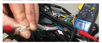
Disconnect the pressure transducer relay harness Measure the supply voltage between the pin 1 and 3 Check that the voltage value is 5 V DC ±5%
